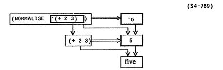
Finally, a slightly more complex case. In the following, <E1> is not in normal-form; it is the xcons redex (xcons 'nth '1 ''[KEEP ON KEEPING ON]). Thus <E1> designates a <T1> that is the nth redex (nth 1 '[KEEP ON KEEPING ON]), which in turn designates an <R> that is the atom KEEP. The normal-form designator of this atom — the example's <T2> — is the handle 'KEEP. Hence <E2>, the normal-form designator of this handle, is the further handle ''KEEP.
